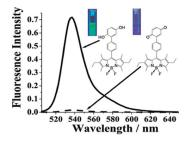
Redox-Controlled Fluorescence Modulation in a BODIPY-Quinone Dyad
